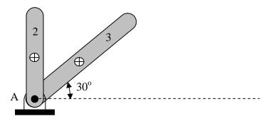
a) What weight is needed to be added at a radial distance 0.5 m from point A (magnitude and orientation) in order to balance the links?
